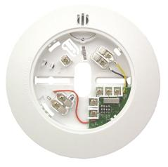
The F220-B6RS 24 VDC Four-wire Detector Base with Sounder meets the requirements of UL464 for a notification device and works with the F220 Series Photoelectric Smoke and Heat Detectors. Power the sounder from the control panel's NAC circuit or from auxiliary power.
